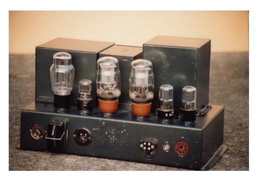
1950. A *Williamson* amplifier marketed by Goodsell, England. This variant incorporates an auxiliary rectifier 6X5 valve (2<sup>nd</sup> from left) for powering attached pre-amps etc.
