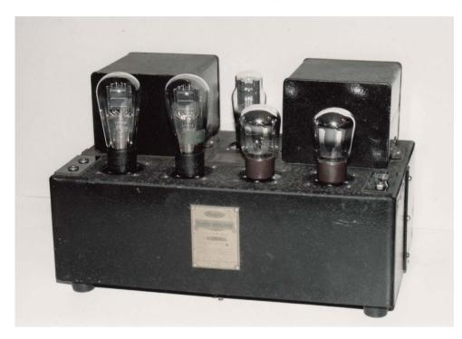
1930. A robustly built early audio amplifier by EMMCO, Australia. Push pull triode output with interstage transformer drive.The output is at high impedance requiring a loudspeaker with its own transformer. 4-5 watts.
