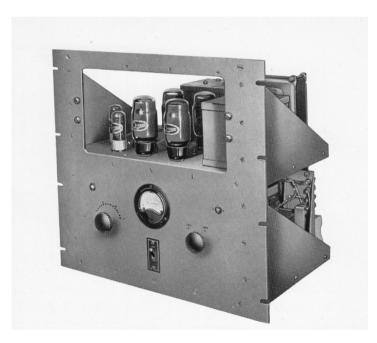
**1945.** An experimental 30 watt amplifier designed by D.T.N.Williamson for the Marconi Osram Valve Co. using four KT66 valves triode connected. From 'Art & Science in Sound Reproduction'. Hugh Brittain 1953.
