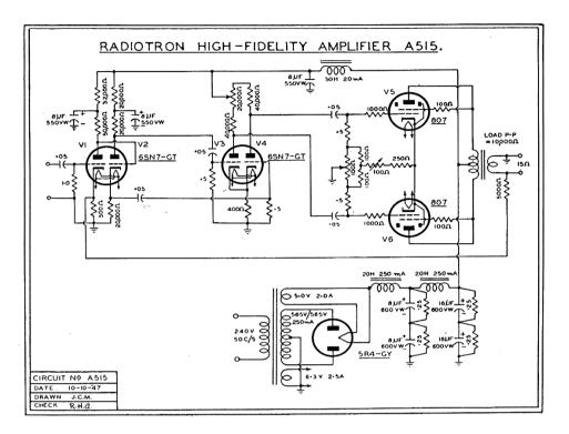
1947-8. The A515 circuit format of the *Williamson* amplifier as developed by the AWV Laboratory, Sydney, with double triode 6SN7 valves for input and type 807 valves for the output stage. It is functionally essentially identical to the original.
