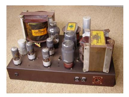
1949. A superbly constructed *Williamson* amplifier of the early format using four type 6J5 valves for the input stages, made by Rogers Developments, England.
