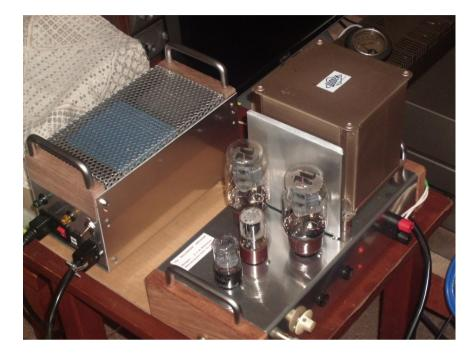
A recently built Williamson amplifier with separate power supply. The output transformer is by Woden (U.K.)
